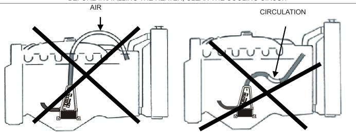
TO AVOID SIPHONS BEING PRODUCED; THERE SHOULD BE NO CURVES IN THE FLEXIBLE TUBES.
