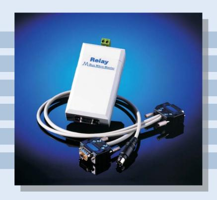
The M-Bus Micro-Master has specially been designed for mobile service. In combination with a laptop it is suitable for setup of individual M-Bus slaves during installation and also for fast and easy reading of small M-Bus systems by external service personnel.
