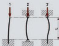
Determine, in the diagram (calculated with safety 1), with the corresponding load case (1 / 2 / 3), the intersection of the buckling force  $F$  and free spindle length  $L$ . The intersection point must lie below the boundary line of the chosen spindle diameter. If not, a bigger spindle, respectively, the next larger gear-box is to be selected.
