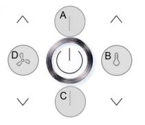
The configuration menu is activated by simultaneously pressing the buttons "up" (A), "left" (D) and "right" (B) for at least 3 seconds.
