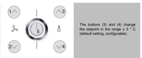
With power-button (5), the device can be set in standby mode by pressing the button (if keycard-switch is NOT used). If the button is used as a occupancy button, the button must be pressed for at least 3s, in all other cases, a short actuation is sufficient. In standby mode, the display and all outputs are switched off (controller deactivated). The frost and heat protection monitoring remains active.
