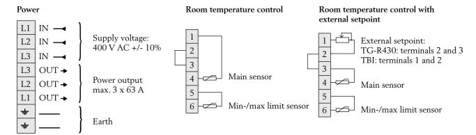
NOTE: When controlling Y-connected loads, the load must be symmetric and the signal neutral must not be connected!
