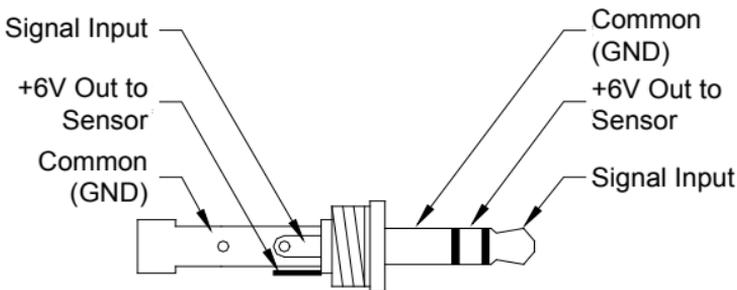
**Figure 2 Input Connector Detail (Stereo plug)**
