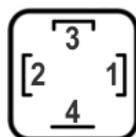
The coil is connected between pins 1 and 2 and in the supplied harness is properly wired to the A connector of the Electronic Sensor.
