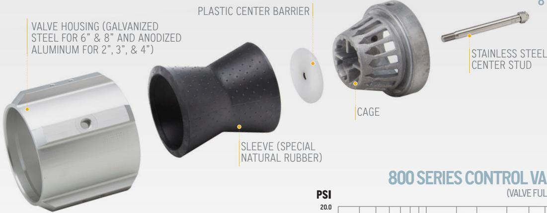
AS A HYDRAULICALLY OPERATED SLEEVE-TYPE VALVE, THE 800 SERIES CONTROL VALVE IS DESIGNED FOR VERSATILITY. THE BASIC BODY CAN BE EQUIPPED WITH SEVERAL DIFFERENT OPTIONS FOR CONTROLLING PRESSURE AND FLOW IN PIPING AT THE PIVOT POINT OR END GUN VALVE CONTROL. IT'S ALSO ENGINEERED FOR EXTREMELY HIGH EFFICIENCY, RESULTING IN LOW PRESSURE LOSS AND HIGH FLOW CAPACITY.
